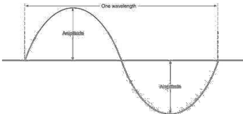
A **cycle** is one complete wave action. The **frequency, measured in Hertz**, is the number of cycles passing a given point in one second.
